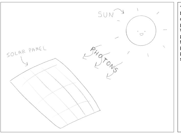
"This rotation is important because solar panels collect energy called photons from the sun. When solar panels are placed near other objects that create shade, the photons won't hit the panel. This renders the solar panels useless."
