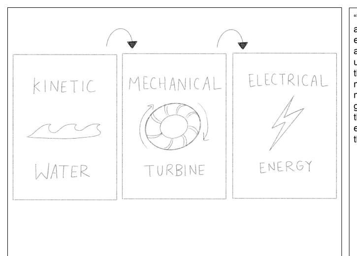
"Well this boat will be another combination of energies. Hydropower and solar! Hydropower uses the kinetic energy of the water and the turbine makes that into mechanical energy. A generator on the boat then turns that into electricity which powers the trash collector."
